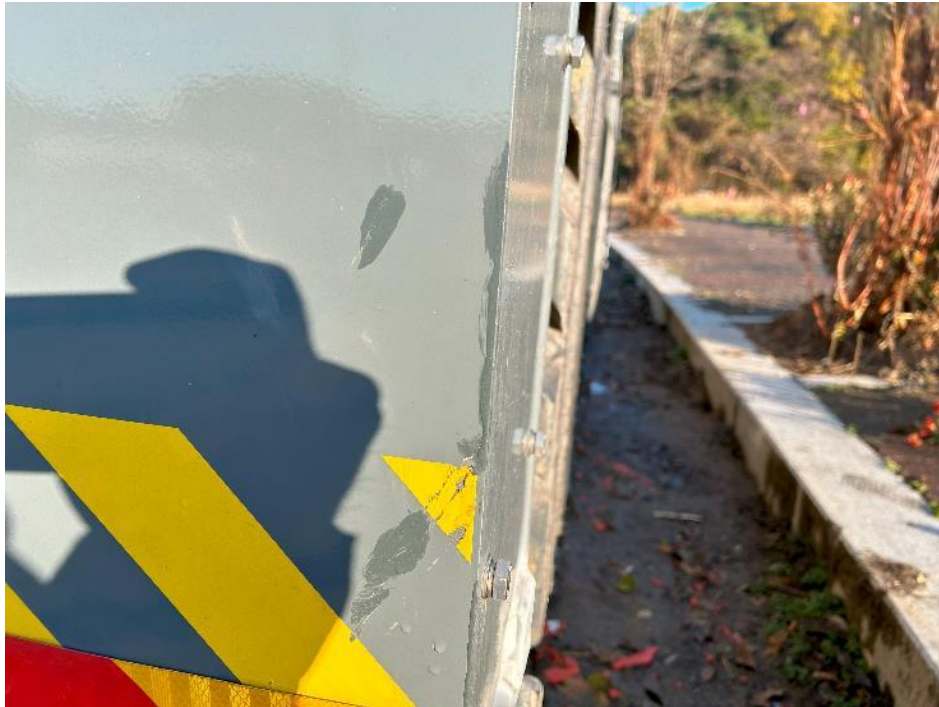
Minor Paint Scratches – touch up covered.
