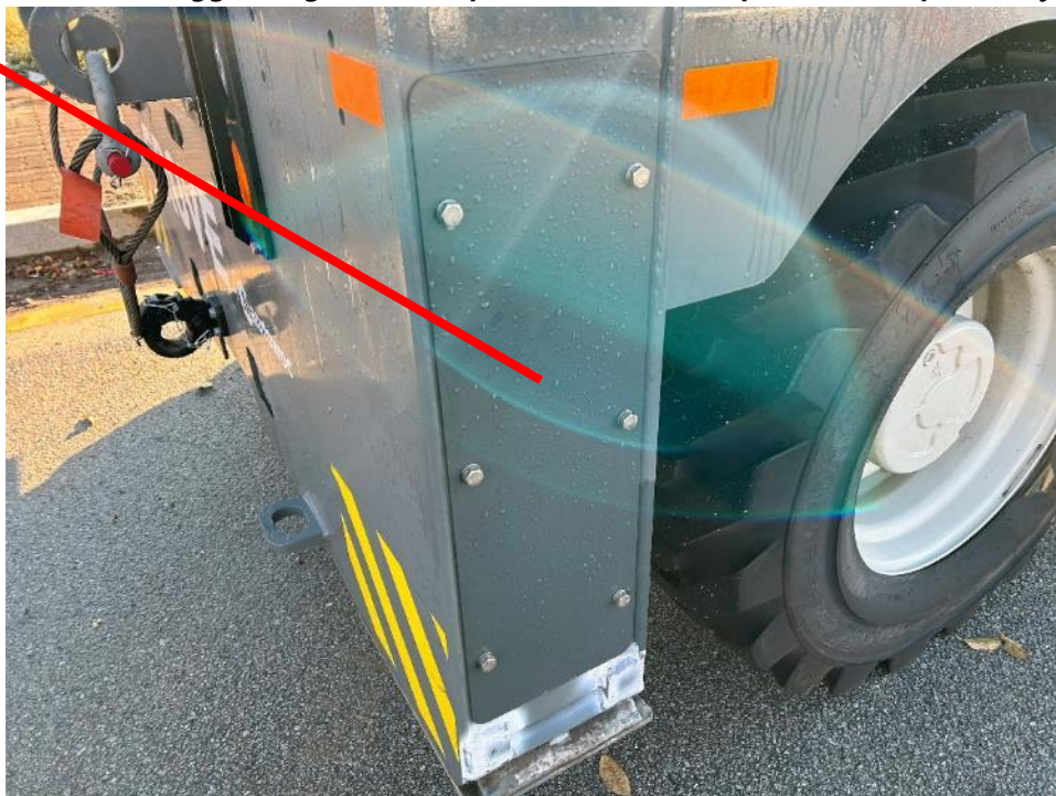
Replaced Part – LH front outrigger original cover plate dented. local produced, replaced by customer.
